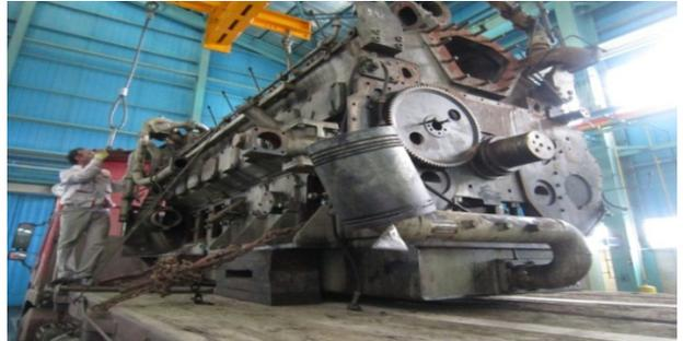
The stage of disassembly and receiving repair engines
