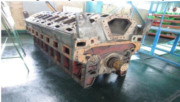
Disassembled engine block
