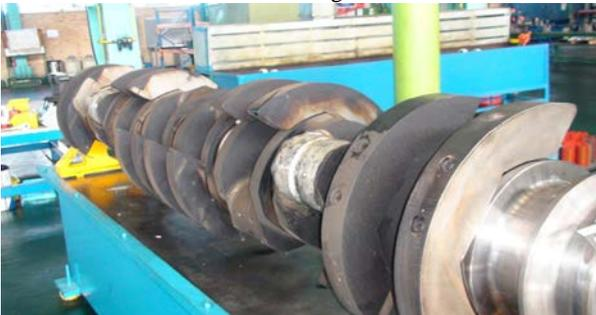
The stage of cleaning all bearing seating surfaces and crankshaft oil drillings
