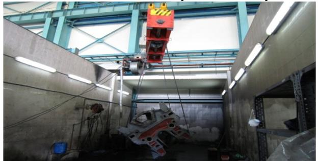
Engine block turnover tool to wash and inspect different sections
